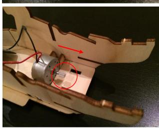
Place the motor in its place when the wire are facing up. Make sure the hinge (cog wheel) are facing the back side of the racer.
