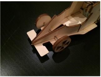
Twist the 2<sup>nd</sup> wheel onto the rod. Use the table to pressure the part in. make sure NOT TO endanger your hand by placing it on top of the rod and pushing down. Use a bit of glue if the wheels are not set on the rod.
