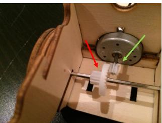
This part is extremely important. If you do not assemble it correctly, the racer is going to drive backwards.
