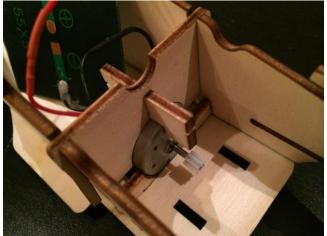
Use the part we just assembled to cage the motor in its place. Slide the part from the top all the way to the bottom.
