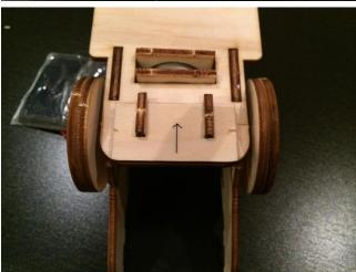
Use the arrow to mark the direction, slide it from the back towards the motor
