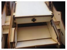
Then the smaller part with the cross crack. Make sure this part is glued correctly and properly.
