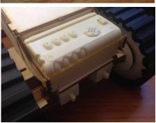
Hold the control box with the rubber band.
