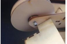
The large wheel goes in the front. Let the kids use the 30 screw they just took out of the wheel. Hand the kids a nylock locknut and a plastic wrench. The screw comes from the outside, and the nylock from the inside. Make sure after the students tighten the screw that the wheel can spin freely.
