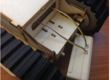
Pull the wires through the model and connect them to the control box, Explain to the kids that if their model is going backwards they can just switch the wires.
