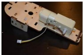
Place the motor. Notice that the cable comes out of the left side.
