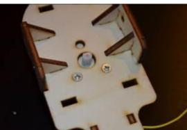
Insert the drilling screws on the other side.
