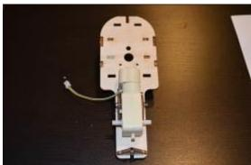
Insert the 30 screw from one side of the motor to the other. Now, the motor is connected to the card. Close and tighten with a locknut.
