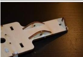
Glue the motor's base and the back triangle.
