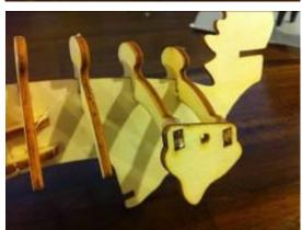
Glue these ribs so that the walls' sticking out sides face backward, as shown in the photo!
