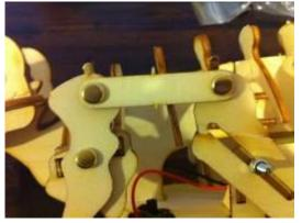
File parts remaining. Connect wooden piece using a paper fastener. Connect arm's top hole to leg's top hole.
