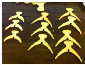
Disassemble and carefully file ribs.
