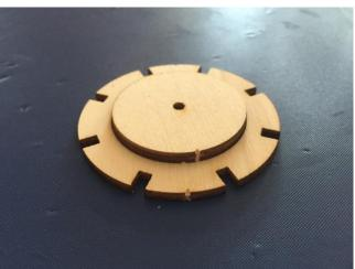
Glue the smaller part onto the larger one, use the round mark on the larger part to place the parts correctly.
