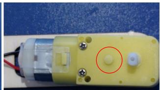
Place the motor in its place. Make sure the bump is facing up (circled in red)
