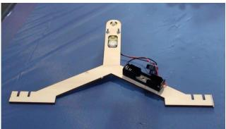
Place the double side tape on the battery box and place it as shown in the picture.
