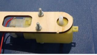
Lock the screws with 2 regular locknuts
