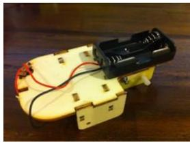
Straighten the cables, and glue them under the servo. Notice that the servo's backside gets to the wood's tip. Otherwise, the dinosaur's balance will be off.
