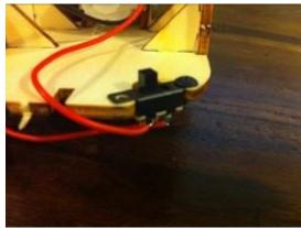
Insert the switch to its place carefully in order not to rip the cables. Hand each student a bug screw, and screw the switch to its place.
