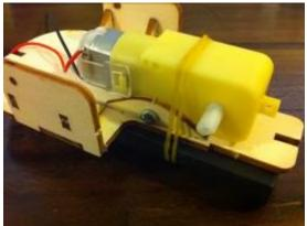
Then, stretch the rubber band previously removed from the servo around the battery place and servo in order to protect the gluing.
