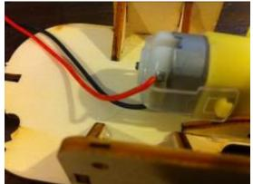
Place servo with the cables on the left, and the red cable on top. Remind students the rules for connecting the servo. After placing the servo, go by each student and make sure they did so correctly.
