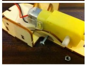
Insert screw from one side of the servo to the other. Tighten with the locknut. It's better to use a screwdriver.
