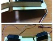
Each servo is connected with 2 servo screws ("10 screw"= 1 cm) and 2 regular locknuts. You may let students assemble on their own by looking at an assembled model. Tighten the screws well using locknuts in order to prevent unnecessary movement of the servo.
