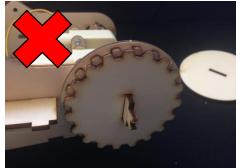
Insert the 2<sup>nd</sup> cog wheel. Make sure both wheels align, if not turn the wheel around.
