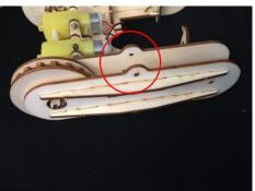
Take the side wall part we glued in the previous lesson and Glue the side wall, and lock the cog wheel in its place. Make sure NO GLUE touches the cog wheel.
