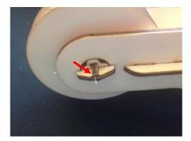
With a small drop of glue, glue the "hill" part on the tip of the hinge (look at red arrow)
