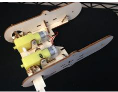
Glue one wall to the side of the base. Make sure the parts are inserted all the way with no spaces between the parts.
