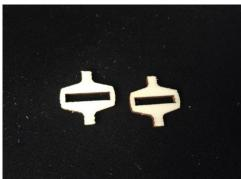
CAREFULLY, break and file the parts as shown in the picture.
