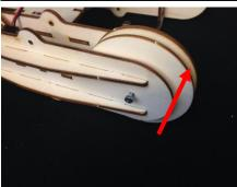
The large wheel goes in the front. Let the kids use the 30 screw they just took out of the wheel. Hand the kids a nylock locknut and a plastic wrench. The screw comes from the outside, and the nylock from the inside (red arrow). Make sure after the students tighten the screw that the wheel can spin freely.
