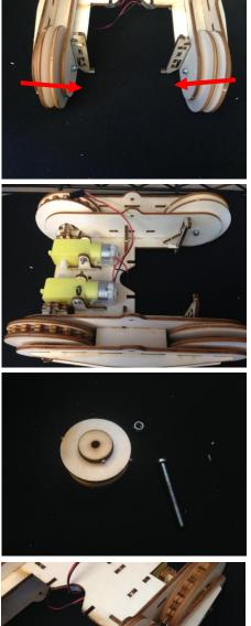
After finishing both large wheels, assemble the small wheels in the middle. Check the directions of the 30 screws (red arrows)
