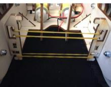
Slide the control box in and secure with the rubber bands
