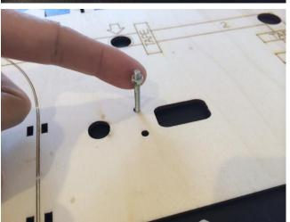
Make sure the gate is still facing the table. Push the screw from the bottom side upwards, so we see the screw on the back side. Place a locknut on the screw
