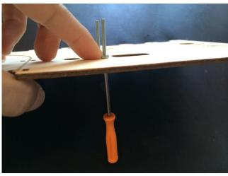
After finishing, hand the kids screwdrivers and tighten up the locknuts.
