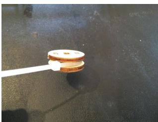
Wrap the zip tie around the wheel and tighten it
