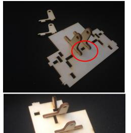
The 2 parts with the claws are glued in the middle
