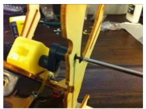
Place the leg's large hole on the crank.
