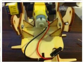
Tighten locknut well, then release a full turn. Check students' work. Then, distribute another screw and locknut, and do the same with the other leg. If connected correctly, legs should be able to stand on their own.
