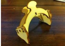
Glue ribs in their place using the walls. Notice that walls are parallel to each other as shown in this photo.
