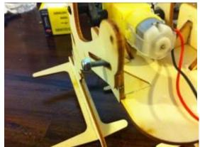
Insert screw from card's wall to diagonal hole of leg. Tighten with a nylock locknut.
