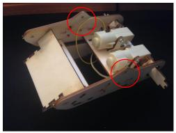
Glue the parts you just filed to the sides of the tank.
