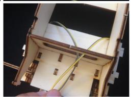
Push the wires to the inside, and slide them through the crack on the bottom side.
