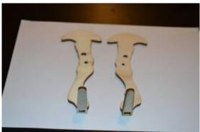
Glue the legs' bottom. Notice that legs should be opposite to one another. Place the legs on the table with the longer sides of the semi-circles on top facing away from one another.
