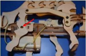
Connect the legs to the card, with the long side of the leg's top semi circle facing backward. Place each large hole on a large hole, and connect the leg to the crankshaft with a drilling screw. Connect the middle of the leg with a paper fastener.
