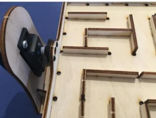
Carefully push the servo head onto the servo.
