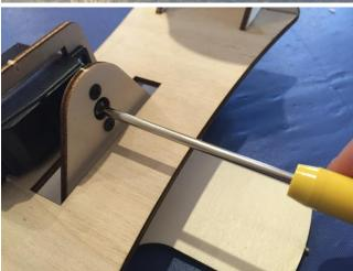
Insert the bug screw from the other side of the triangle part, straight into the servo through the servo head.
