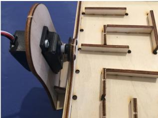
Take the maze plate, align the servo head and the servo together.
