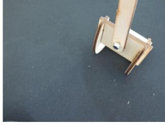
Place the long bar behind the chair, insert the screw and tighten it with the locknut.
