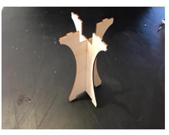
Apply glue in the cracks and slide the parts together.
