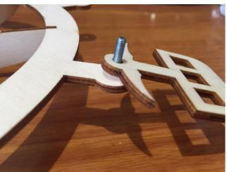
Place the cart on top of the large wheel (not under), insert the screw from the bottom part and lock it with the Nylock from the top.
