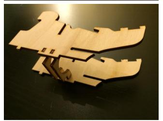
Sandwich the gate parts with the walls (make sure the walls and the gates are symmetrical)
