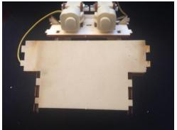
Glue it to the front side of the body. Make sure the kids apply enough glue and inserted the part to its proper place.
