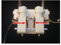
Hand the kids a 30 screw and a lock nut, The 30 screws come from the outside and the nuts from the inside.
