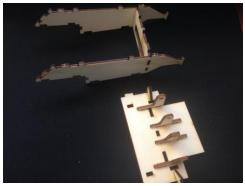
Glue the middle part in between the walls (there's only one way to glue it correctly)
