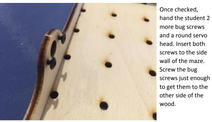
Place the servo head from the outer side of the wall. Align it so the screws meet only middle holes (like shown earlier in this lesson plan)
