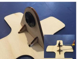
First, screw the bug screws just enough to get them to the other side of the wood. Then place the servo head in its place, only then one by one tighten the screws.
