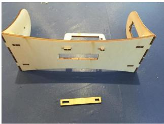
Once all the students inserted the "gate" part tilt the model on its side, and glue the rectangular part onto the bottom of the "gate" part.
