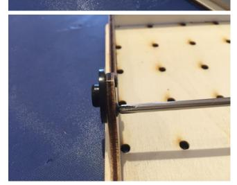
Use a screwdriver to tighten the screws into the servo head.
