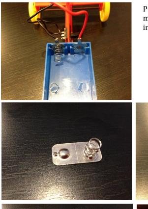
Put the red and black wires' metal parts in their places inside the battery box.
