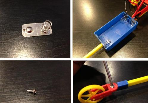
Hand each student the part shown in the photo. Place it in the other side of the battery box. Each spring should be across from a bump and vice versa.
