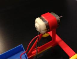
Hand each student a propeller and place it on the motor's hinge.
