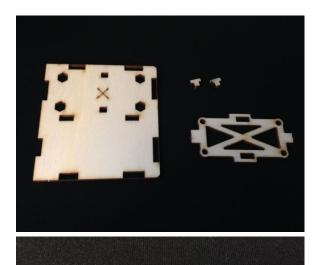
After painting and drying the wooden sheet, break down and file the parts as shown in the picture.
