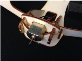
Using a little glue, place the part above the motor, and make sure it is inserted all the way.
