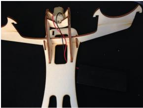
Carefully, place the motor in its place, see that the hinge is facing outside)
