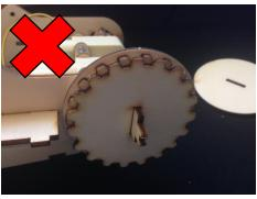
Insert the 2<sup>nd</sup> cog wheel. Make sure both wheels align, if not turn the wheel around.
