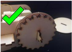
On this picture we can see the proper insertion of the second cog wheel.
