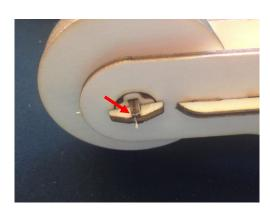
With a small drop of glue, glue the "hill" part on the tip of the hinge (look at red arrow)
