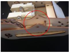
Glue the side wall, and lock the cog wheel in its place. Make sure NO GLUE touches the cog wheel.
