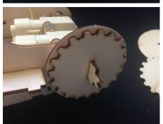
Take 1 cog wheel and insert it onto the hinge.
